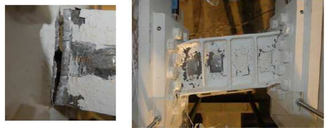
Fig. 11 Fracture at the bottom left flange and final deformation of link specimen JPN
