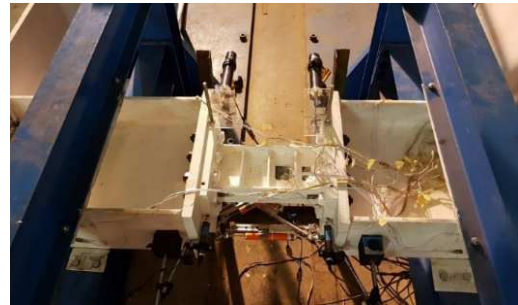
Fig. 21 Link to coupling beam connection before testing
