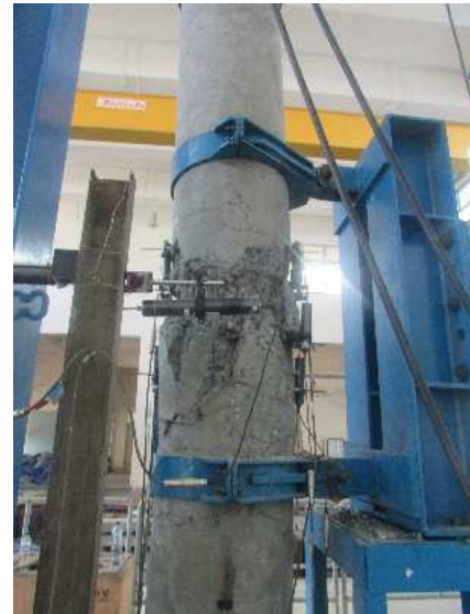
Fig. 11 Totally explosion damage of specimen S-TB-3
