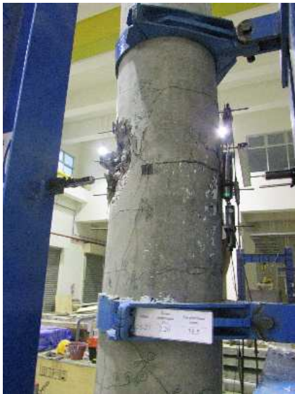
Fig. 10 The crushing on the front and the rear face of specimen S-TB-1
