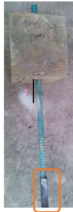
Fig. 5 Grip of GFRP Specimen
