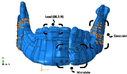
Fig. 1 Loading and boundary condition setup in simulation
