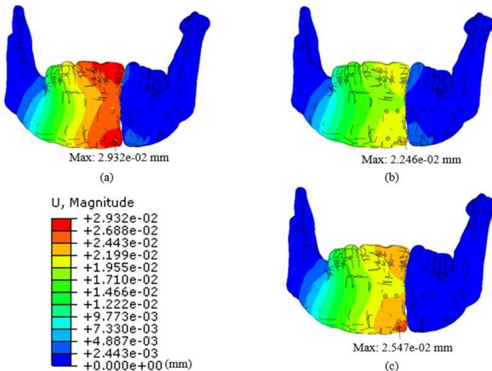
Fig. 2 Displacement of along the system from (a) MF-24, (b) MF-44, and (c) MF-42
