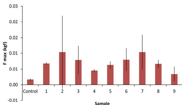
Fig. 8 Maximum load to deform the green grass jelly
