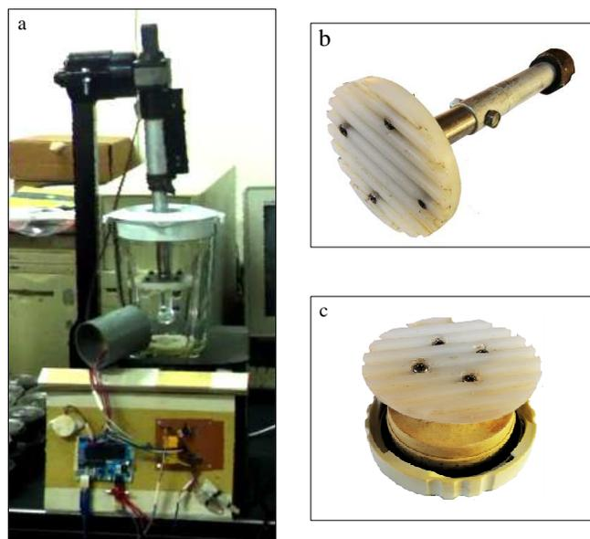
Fig. 4 (a) Complete structure of semi-automatic green grass jelly squeezer, (b) Upper squeezer (c) Bottom squeezer
