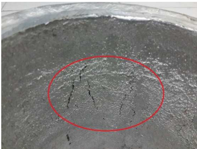
Fig.10 Cracks that occur in the cast part with direct contact with the mold core
