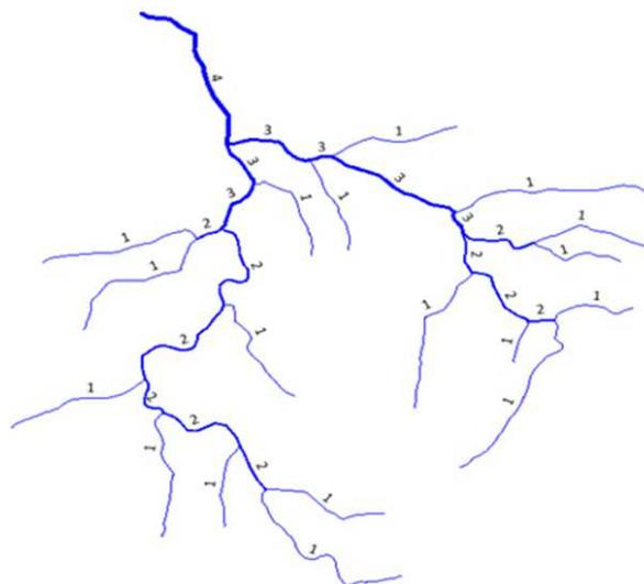
Fig. 2 Determination of stream order by segmentation method [23].
