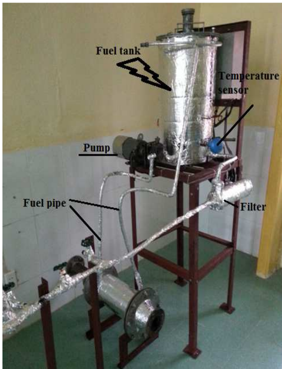
Fig. 1. A heating fuel supply system
