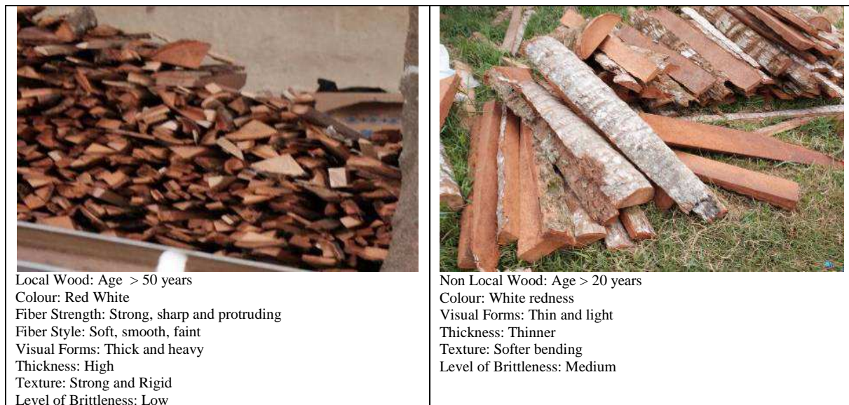
Fig. 2 Characteristic of wood coconut waste
