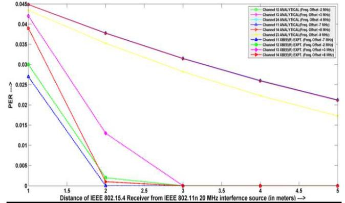
Fig.14: Packet Error Rate of IEEE 802.15.4 (Zigbee™) in the presence of interference Source IEEE 802.11n HT 20MHz OFDM (2402-2422MHz) Channel 1: (Center Frequency at 2412 MHz)
