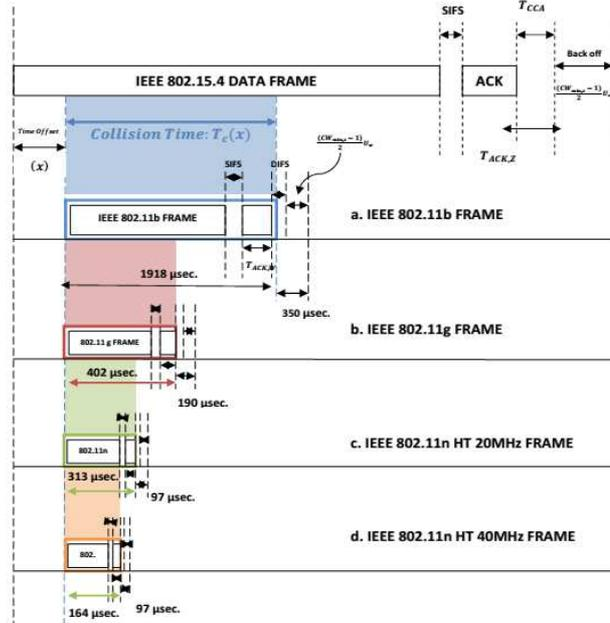
Fig.8: Collision Time  $T_c(x)$  for overlapping frames of different IEEE 802.11 standard and IEEE 802.15.4 frame with a varying time offset 'x'
