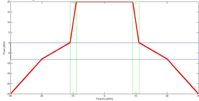
Fig.6 (b). Transmit Spectral mask for IEEE 802.11n HT 20MHz simulated in MATLAB [Distribution of PSD]
