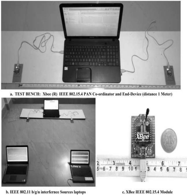
Fig.10: Experimental setup for finding out Packet Error Rate (PER) of IEEE 802.15.4 (XBee® Zigbee Modules) in the presence of interference from IEEE 802.11 b/g/n Network
