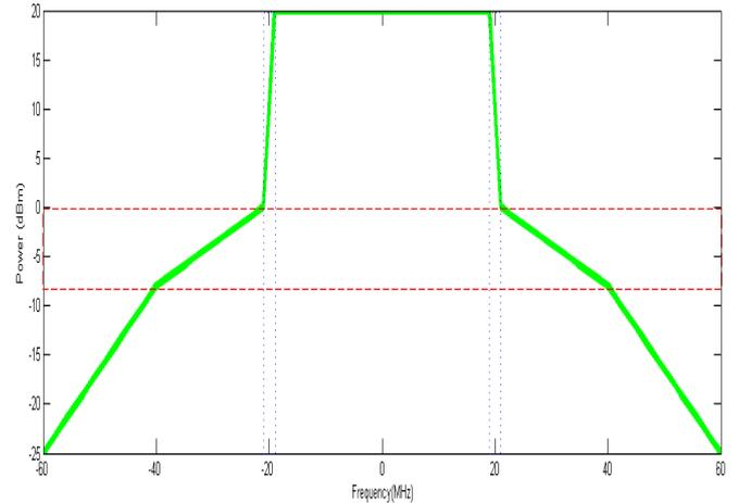
Fig.7 (b). Transmit Spectral mask for IEEE 802.11n HT 40MHz simulated in MATLAB [Distribution of PSD]
