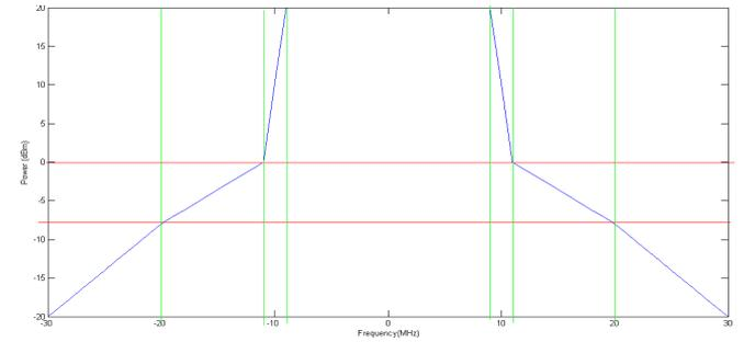
Fig. 5 (b). Transmit Spectral mask for IEEE 802.11g simulated in MATLAB [Distribution of PSD]
