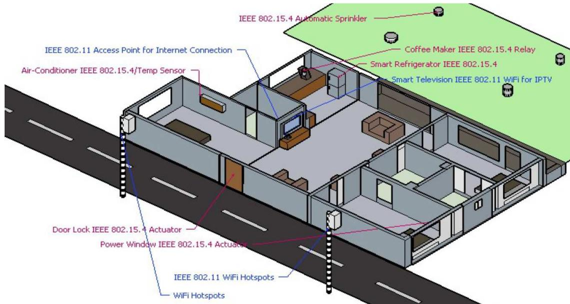
Fig.1 Internet of Things deployment using heterogeneous wireless Networks
