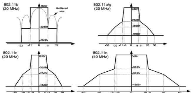
Fig.3 Transmit Spectral Mask for IEEE 802.11 b/g and IEEE 802.11n (20 MHz and 40 MHz Channel) [8]
