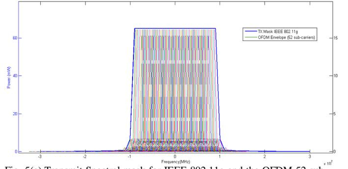
Fig. 5(a). Transmit Spectral mask for IEEE 802.11g and the OFDM 52 sub-carrier envelope simulated in MATLAB [Distribution of PSD]
