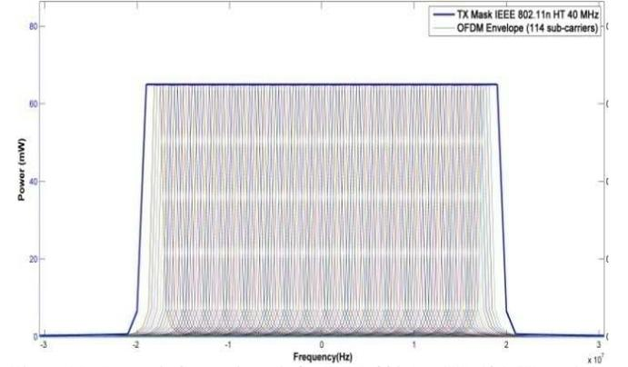
Fig. 7 (a). Transmit Spectral mask for IEEE 802.11n HT 40 MHz and the OFDM 114 sub-carrier envelope simulated in MATLAB [Distribution of PSD]
