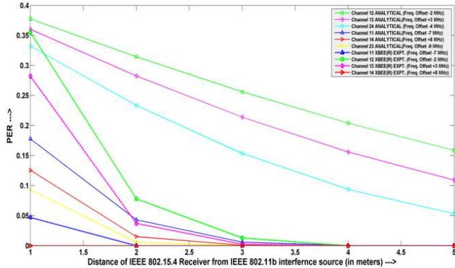
Fig.12: Packet Error Rate of IEEE 802.15.4 (Zigbee™) in the presence of interference Source IEEE 802.11b DSSS 22MHz (2401-2423 MHz) Channel 1: (Center Frequency at 2412 MHz)
