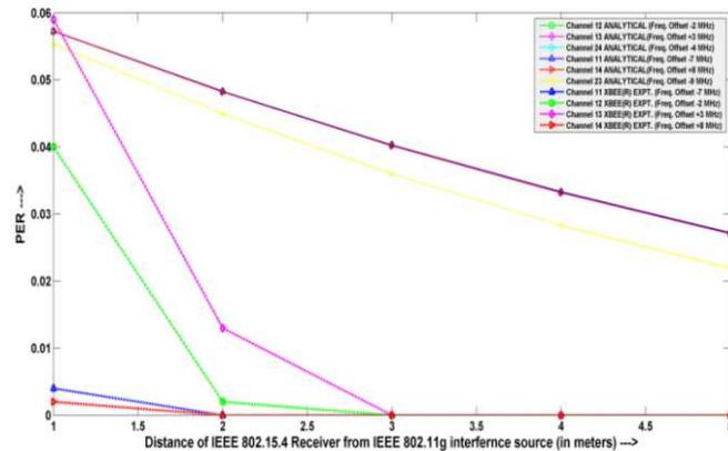
Fig. 13: Packet Error Rate of IEEE 802.15.4 (Zigbee™) in the presence of interference Source IEEE 802.11g OFDM 20MHz (2402-2422MHz) Channel 1: (Center Frequency at 2412 MHz)
