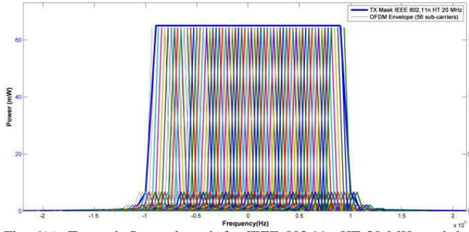
Fig. 6(a). Transmit Spectral mask for IEEE 802.11n HT 20 MHz and the OFDM 56 sub-carrier envelope simulated in MATLAB [Distribution of PSD]
