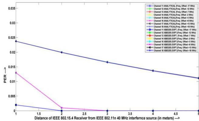
Fig.15 : Packet Error Rate of IEEE 802.15.4 (Zigbee™) in presence of interference Source IEEE 802.11n HT 40 MHz OFDM (2402-2442MHz) Channel 1 + 5 : (Center Frequency at 2422 MHz)
