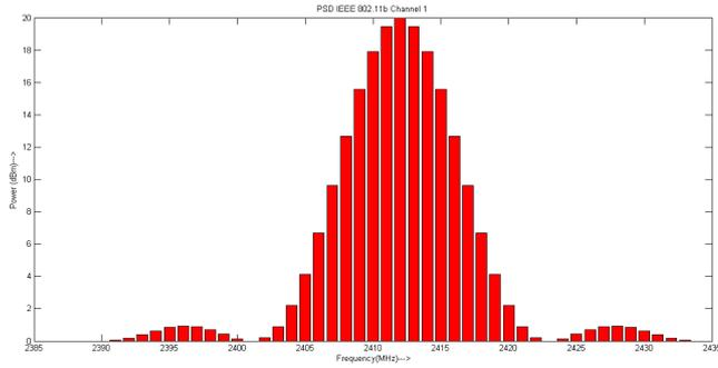
Fig. 4. Transmit Spectral mask for IEEE 802.11b simulated in MATLAB [Distribution of PSD]
