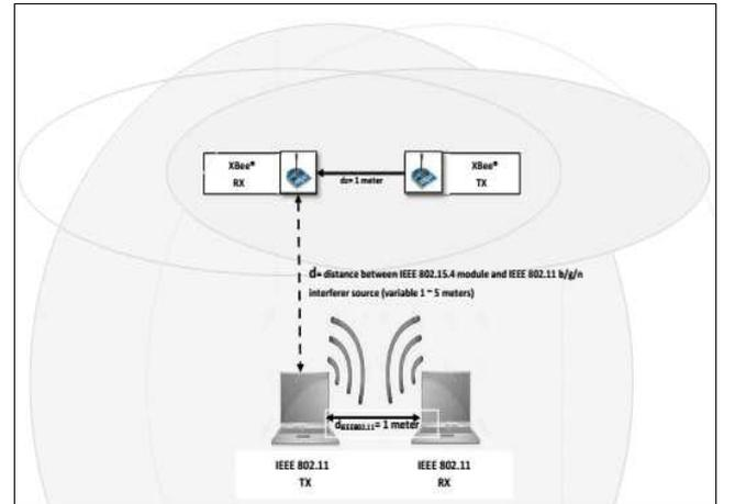
Fig.9: Testbed for measuring PER of XBEE® 802.15.4 under the interference of IEEE 802.11 b/g/n
