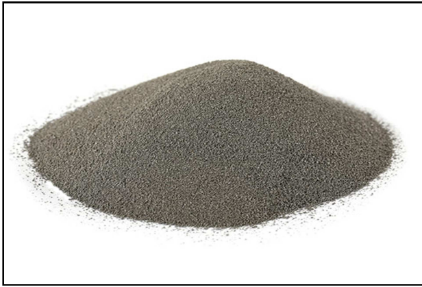
Fig. 2 Iron Powder about 100 mesh (about 150 \mu\text{m} )
