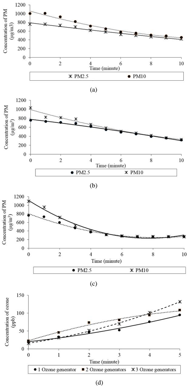
Fig.8. Responses of the sensors during the air purification processes without fuzzy logic control: (a) one ozone generator, (b) two ozone generators, (c) three ozone generators, and (d) clean air condition.
