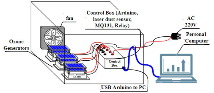
Fig.1 Design of electrostatic air filtration
