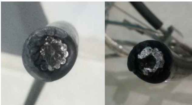
Fig. 7 AAAC-S cross section after the short circuit test
