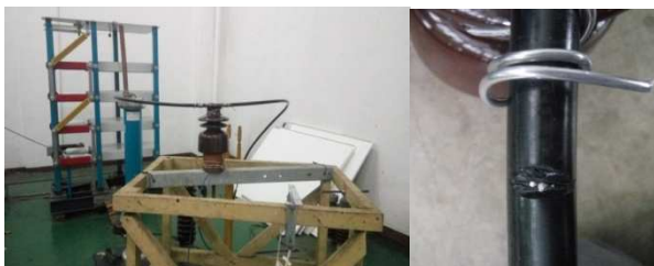
Fig. 4 Voltage impulse testing
