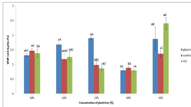
Fig. 1 Water vapour permeability of unripe banana film incorporated with different type and concentration of plasticizer
