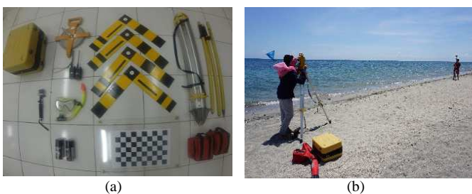
Fig. 1(a) Field equipment and (b) Control Point measurement
