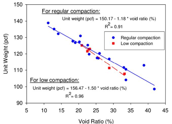
Fig. 9 Effect of improper compaction on concrete weight [19]
