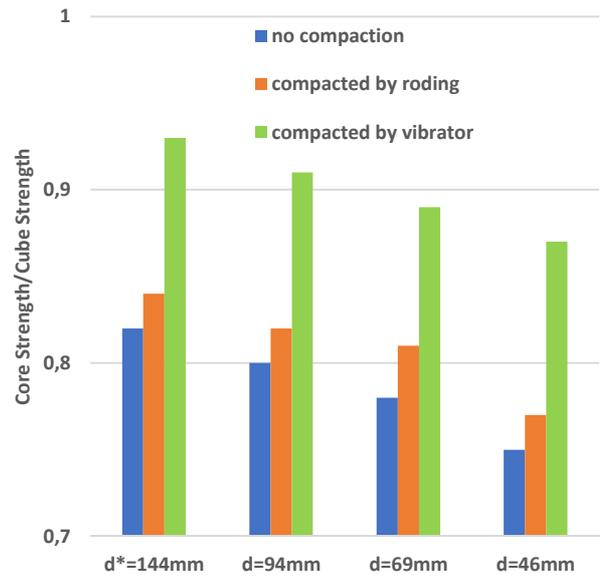
Fig. 8 Effects of compaction [11]
