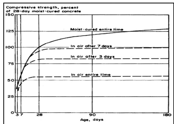
Fig.14 Effects of curing conditions on  $f_c'$  [21]
