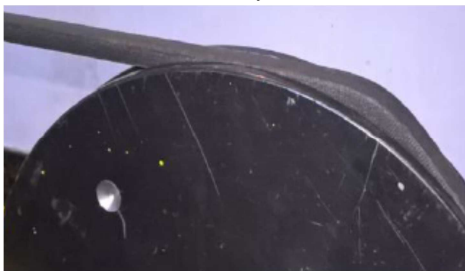
b) Little bump in the driving pulley
