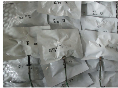
Fig. 4 F 0 -meter measurement inside Rendang Retort Pouch
