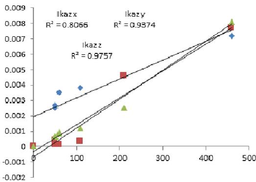
Fig. 5 Correlation between the I-kaz<sup>TM</sup> multilevel coefficient and flank wear at 0.6 mm depth of cut
