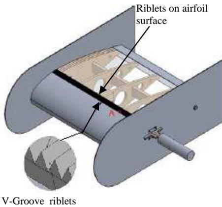
Fig. 1 Location of riblets on airfoil surface [10]
