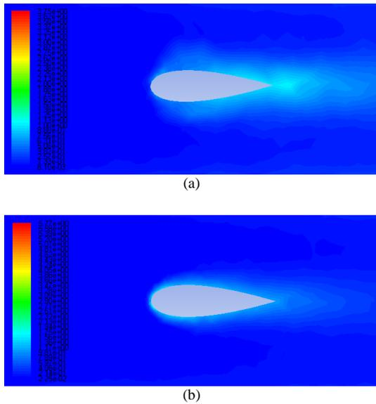
Fig. 7 Turbulent kinetic energy (a) clean airfoil (b) airfoil with riblets
