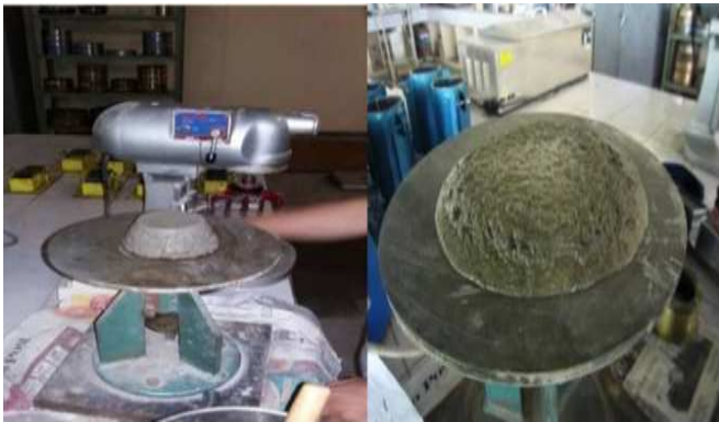
Fig. 3 A flow test to measure the consistency of mortar using a flow table.
