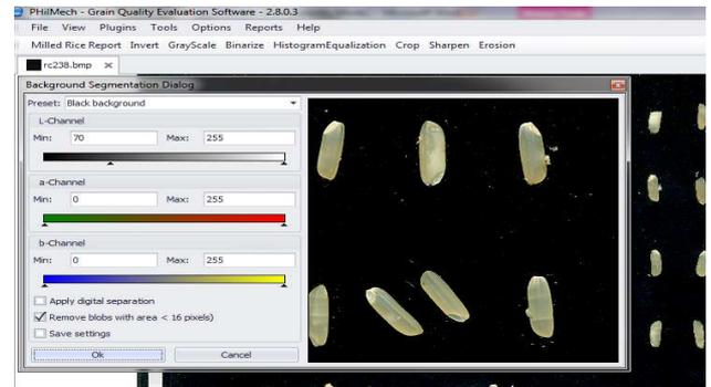
Fig. 5 Menu showing some options for changing the settings of the CVS software
