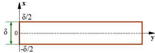
Fig. 3 Flat plate model for drying Ganoderma lucidum
