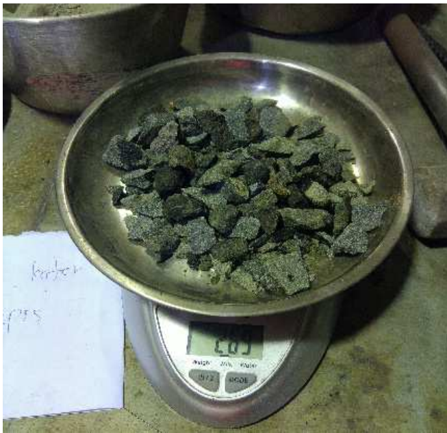
Fig. 1 The ballast aggregate abrasion test process
