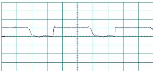
Fig. 11 main switch gate pulse (sampled with oscilloscope)
