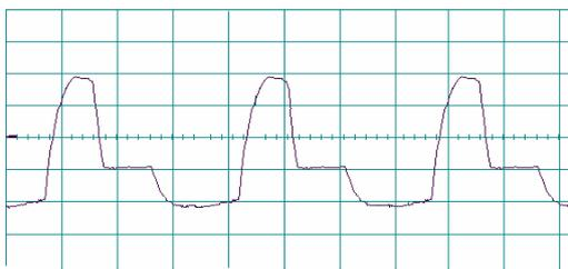
Fig. 10 main switch current (sampled with CT & oscilloscope)
