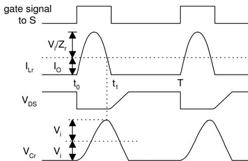
Fig. 3 Waveforms of resonant Dc to Dc step down converter(fig2)
