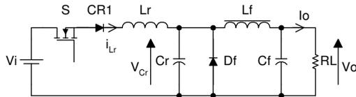
Fig. 2 Resonant step down DC to DC converter
