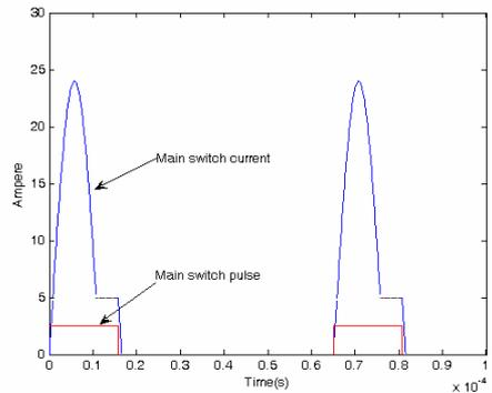
Fig. 8 simulation of main switch current
