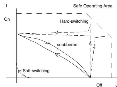
Fig. 1 Switching Diagram(hard switching and soft switching)
