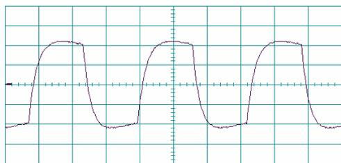
Fig. 12 resonant capacitor voltage (sampled with oscilloscope)
