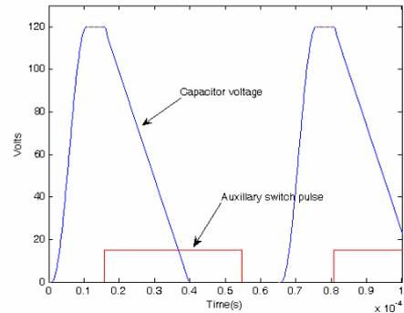
Fig. 7 simulation of resonant capacitor voltage
