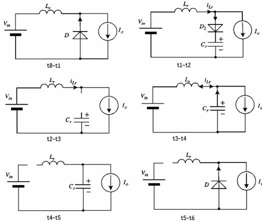
Fig. 5 six intervals of a cycle
