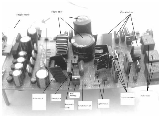
Fig. 9 2 KW prototype
