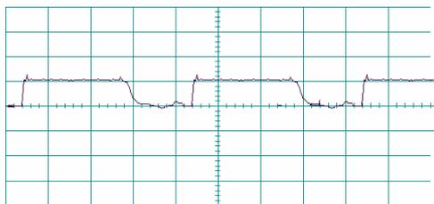
Fig. 13 auxiliary switch gate pulse (sampled with oscilloscope)
