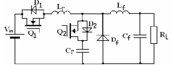
Fig. 4 The plan presented of combining PWM and resonant converters
