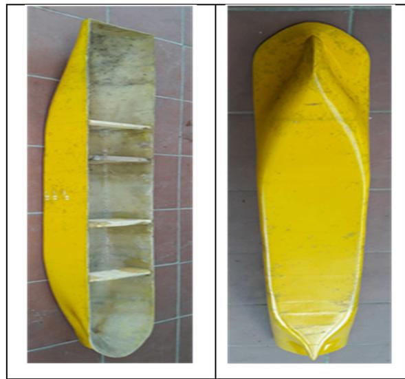
Fig. 7 Image of ship model after fabrication
